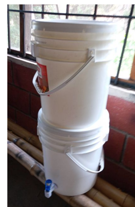
New version of water filter utilizing low cost materials
