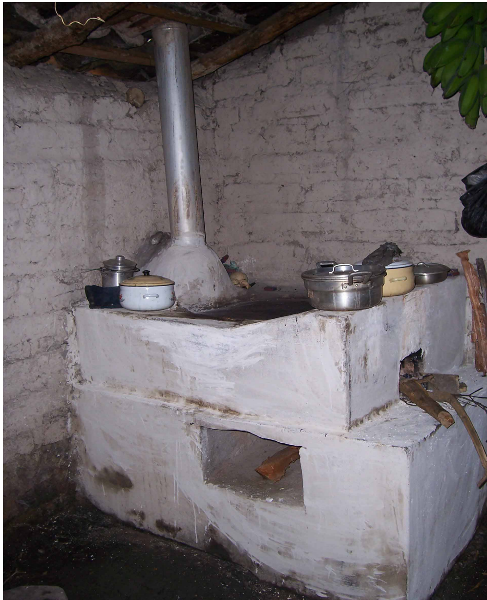
Improved cook stove in operation six months after construction
